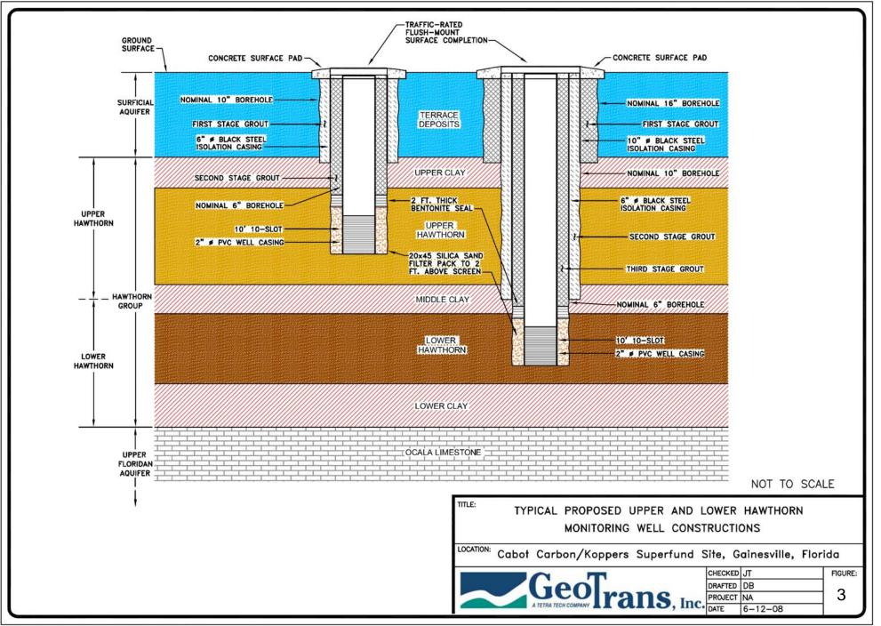
T:\Gainesville\Hawthorn Wells\Work Plan\Revision 3 2008\Fig 2 - typ proposed HG wells.dwg
